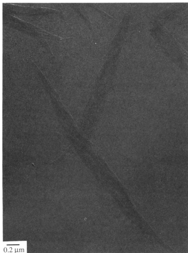
Figure 1. Transmission electron micrograph of sheaves of nylon 4 crystals shadowed with Pt/Pd.
